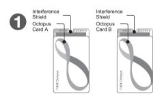
If a user keeps two Octopus cards for different occasions, he/she can use the Interference Shield to separate the two Octopus cards, to avoid interference from one Octopus card while using the other to perform a transaction.
